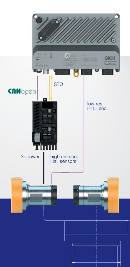
compact. complete. b-drives redundant encoder system
